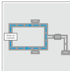
Thinking a step ahead stratojet printers come with an Advance Circulation Technology (ACT), which consist of two functions:
